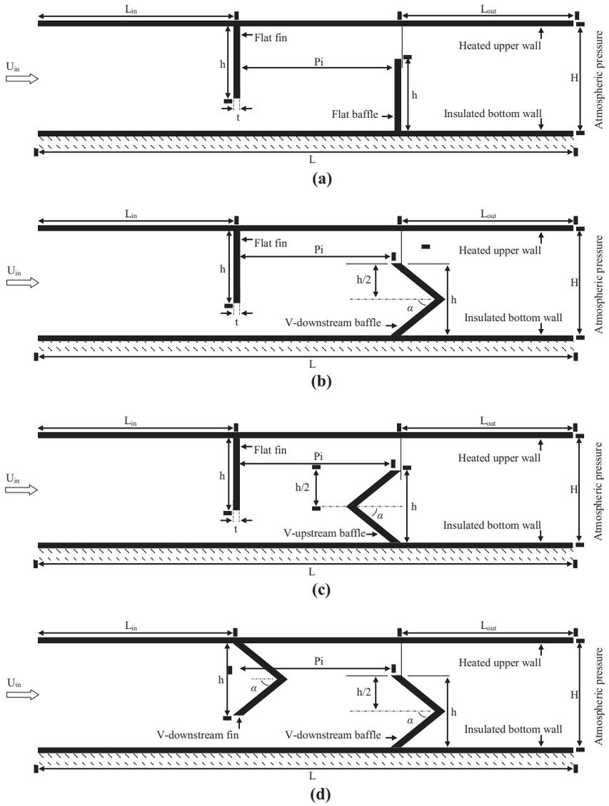
**Figure 1.** The two-dimensional physical model that represents a rectangular channel for various obstacle situations
