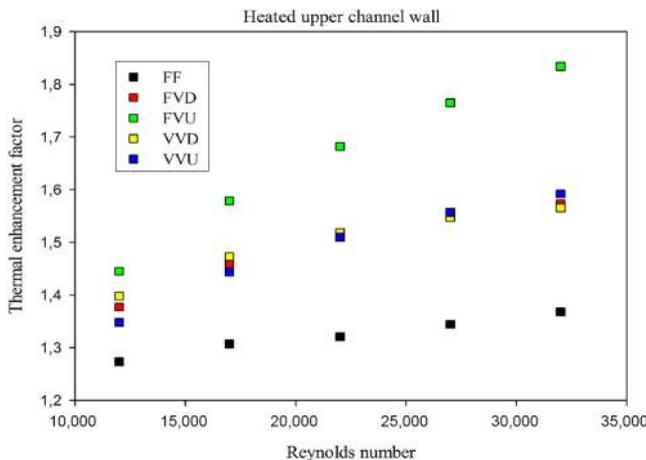
Figure 14. Thermal enhancement factor for various obstacles
