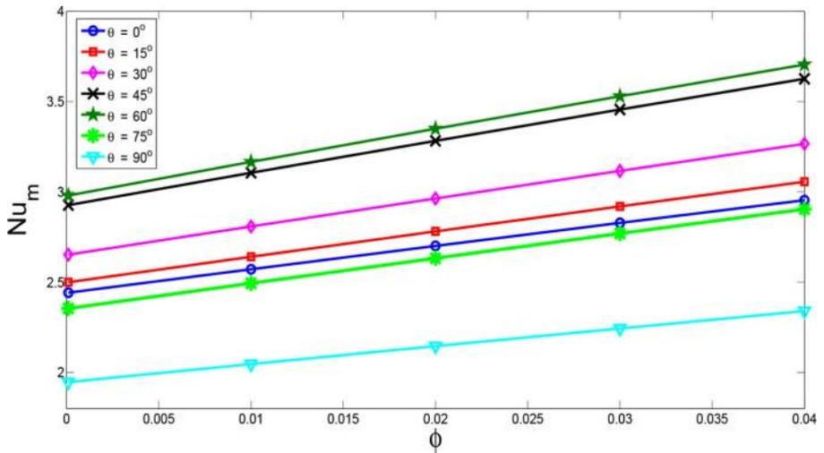
**Figure 6.** Average Nusselt number versus solid nanoparticle volume fraction for different inclination angles of the lower branching channel ( $Re = 300$ ,  $Ha = 5$ )
