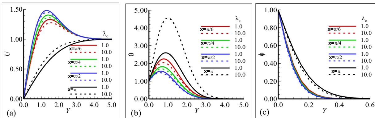
**Fig. 6** Plots of (a) velocity profile (b) temperature profile and (c) mass concentration for  $\lambda_c = 1.0, 10.0$ , when  $\lambda_t = 1.1$ ,  $R_d = 2.0$ ,  $Pr = 7.0$ ,  $Sc = 2.0$ ,  $N_t = 0.5$ , and  $k = 1.0$ .
