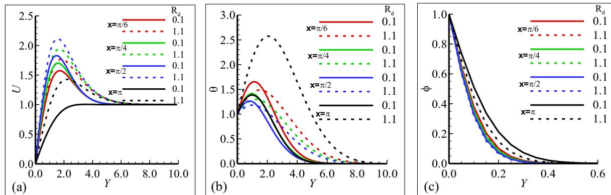
**Fig. 2** Plots of (a) velocity profile (b) temperature profile and (c) mass concentration for  $R_d = 0.1, 1.1$  when  $\lambda_t = 1.1$ ,  $\lambda_c = 1.1$ ,  $Pr = 0.71$ ,  $Sc = 2.0$ ,  $N_t = 0.4$ , and  $k = 1.0$ .
