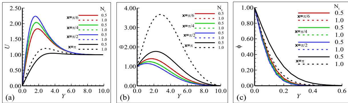
**Fig. 7** Plots of (a) velocity profile (b) temperature profile and (c) mass concentration for  $N_t = 0.5, 1.0$  when  $\lambda_t = 1.1, \lambda_c = 1.1, Pr = 0.71, Sc = 2.0, R_d = 2.0,$  and  $k = 1.0$ .
