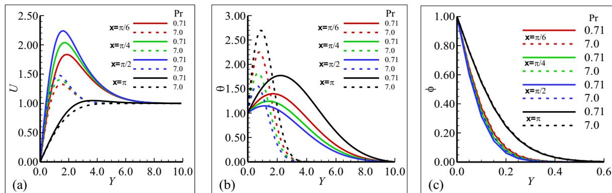
**Fig. 3** Plots of (a) velocity profile (b) temperature profile and (c) mass concentration for  $Pr = 0.71, 7.0$  when  $\lambda_t = 1.1$ ,  $\lambda_c = 1.1$ ,  $R_d = 2.0$ ,  $Sc = 2.0$ ,  $N_t = 0.5$ , and  $k = 1.0$ .
