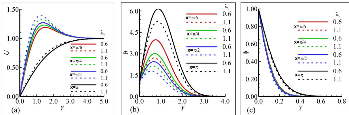
**Fig. 4** Plots of (a) velocity profile (b) temperature profile and (c) mass concentration for  $\lambda_t = 0.6, 1.1$  when  $R_d = 1.1$ ,  $\lambda_c = 1.0$ ,  $Pr = 7.0$ ,  $Sc = 2.0$ ,  $N_t = 0.6$ , and  $k = 1.0$ .
