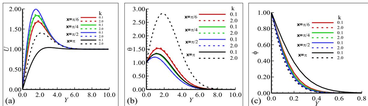
**Fig. 8** Plots of (a) velocity profile (b) temperature profile and (c) mass concentration for  $k = 0.1, 2.0$  when  $\lambda_t = 1.1, \lambda_c = 1.1, Pr = 0.71, Sc = 0.6, R_d = 0.6,$  and  $N_t = 2.0$ .
