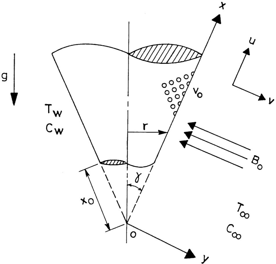
Figure 1. Problem schematics and coordinate system.
