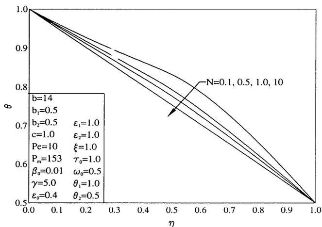
Fig. 7. Effect of  $N$  on temperature distribution
