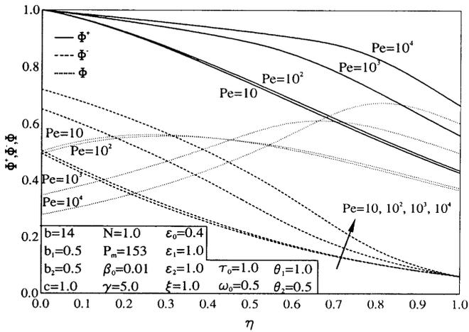
Fig. 12. Effect of  $Pe$  on  $\Phi^+$ ,  $\Phi^-$  and  $\Phi$
