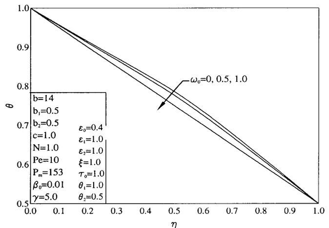
Fig. 5. Effect of  $\omega_0$  on temperature distribution
