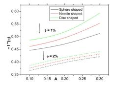
Figure 9. Effect of  $\phi$  and A on skin friction coefficient
