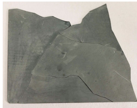
FIGURE 5: Top part of solar cell after removing antireflecting coating (pure silicon).
