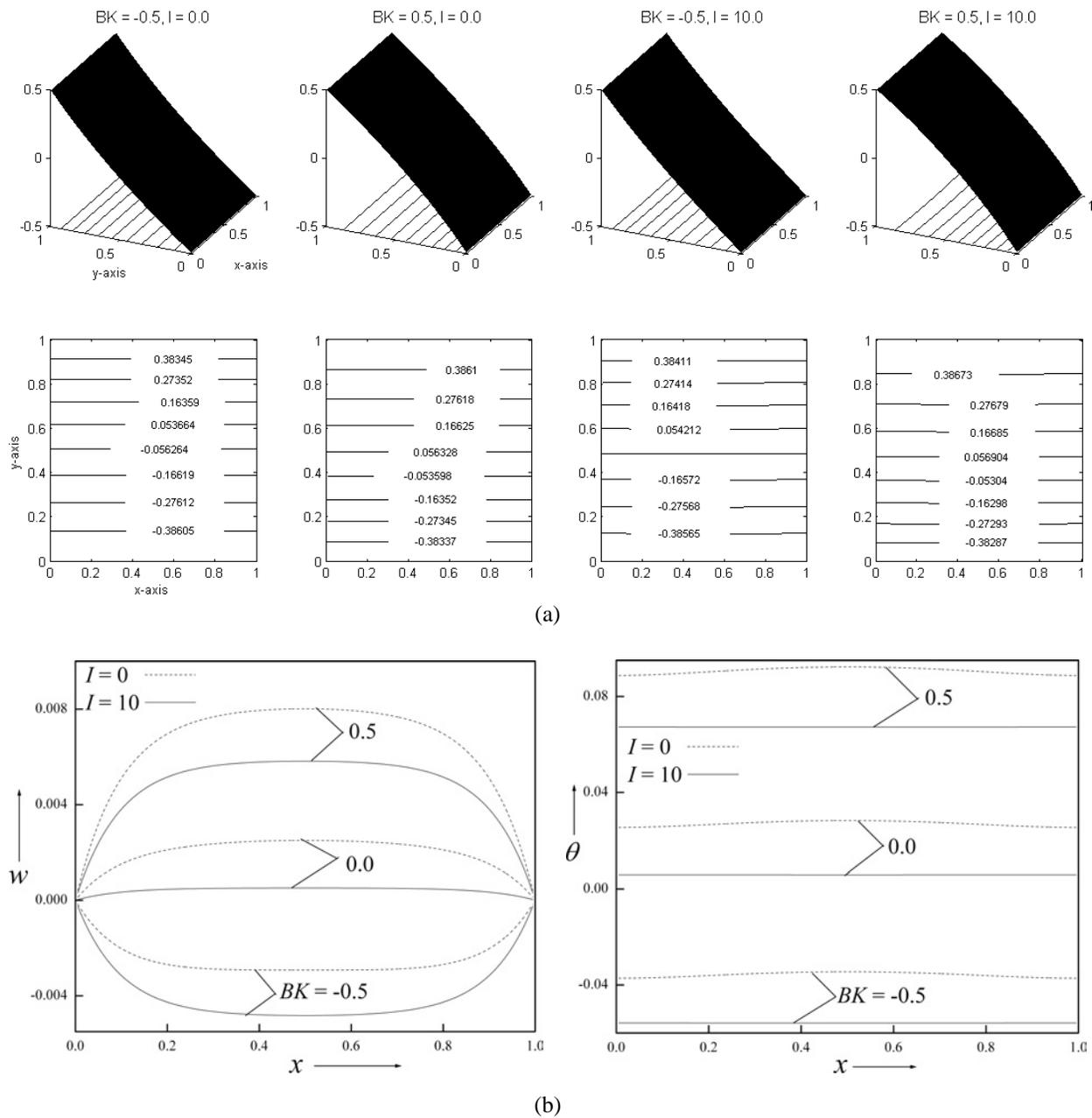
**FIG. 5:** Velocity and temperature contours (a) and velocity and temperature profiles (b) for different values of  $BK$  and  $I$  with  $Gr = 10$ ,  $Br = 1.0$ ,  $Da = 0.01$ ,  $A = 1.0$ , and  $\phi = 0.02$  for copper nanoparticles
