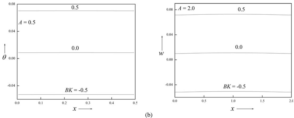
**FIG. 9:** Velocity and temperature contours (a) and velocity and temperature profiles (b) for different values of  $BK$  and  $A$  with  $Gr = 10$ ,  $Br = 1.0$ ,  $Da = 0.01$ ,  $I = 2.0$ , and  $\phi = 0.02$  for copper nanoparticles
