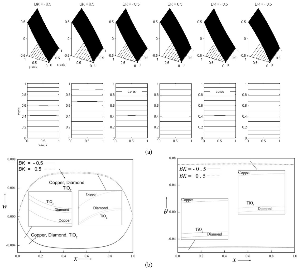
**FIG. 2:** (a) Velocity and temperature contours for different nanofluids and  $BK$  values with  $Gr = 10$ ,  $Br = 1.0$ ,  $Da = 0.01$ ,  $I = 2.0$ ,  $A = 1.0$ , and  $\phi = 0.02$ ; (b) velocity and temperature profiles for different nanofluids and  $BK$  values with  $Gr = 10$ ,  $Br = 1.0$ ,  $Da = 0.01$ ,  $I = 2.0$ ,  $A = 1.0$ , and  $\phi = 0.02$  at  $y = 0.1$
