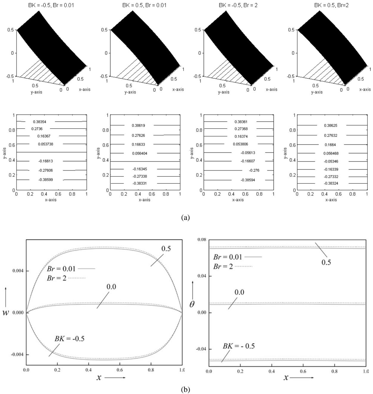
**FIG. 7:** Velocity and temperature contours (a) and velocity and temperature profiles (b) for different values of  $BK$  and  $Br$  with  $Gr = 10$ ,  $Da = 0.01$ ,  $I = 2.0$ ,  $A = 1.0$ , and  $\phi = 0.02$  for copper nanoparticles
