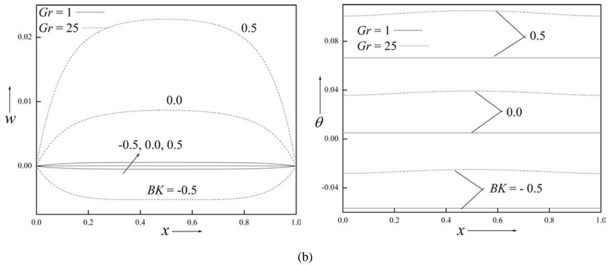
**FIG. 6:** Velocity and temperature contours (a) and velocity and temperature profiles (b) for different values of  $BK$  and  $Gr$  with  $Br = 1.0$ ,  $Da = 0.01$ ,  $I = 2.0$ ,  $A = 1.0$ , and  $\phi = 0.02$  for copper nanoparticles
