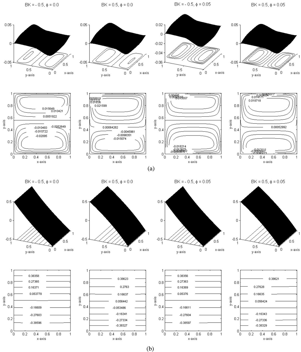
**FIG. 8:** Velocity and temperature contours (a) and velocity and temperature profiles (b) for different values of  $BK$  and  $\phi$  with  $Gr = 10$ ,  $Br = 1.0$ ,  $Da = 0.01$ ,  $I = 2.0$ , and  $A = 1.0$  for copper nanoparticles
