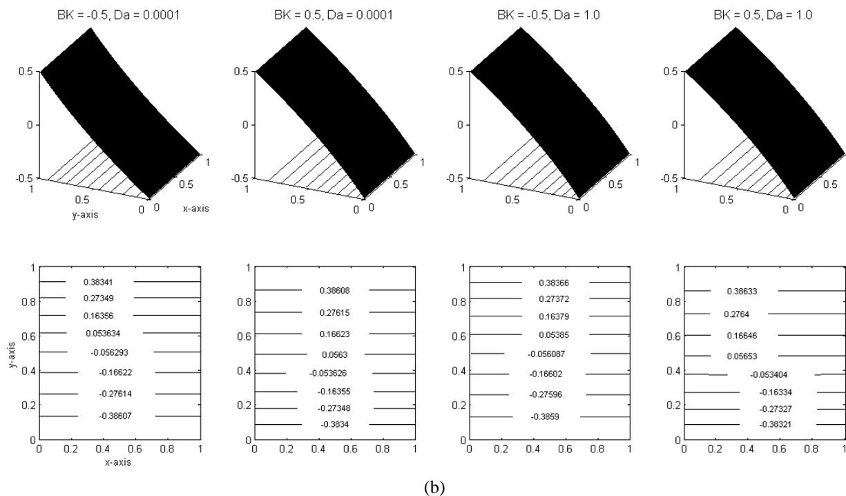
**FIG. 4:** Velocity and temperature contours (a) and velocity and temperature profiles (b) for different values of  $BK$  and  $Da$  with  $Gr = 10$ ,  $Br = 1.0$ ,  $I = 2.0$ ,  $A = 1.0$ , and  $\phi = 0.02$  for copper nanoparticles
